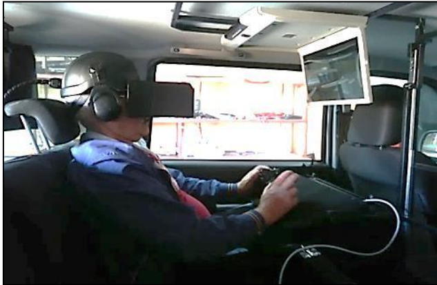
Operator workstation based on polyjoysticks and video headset
